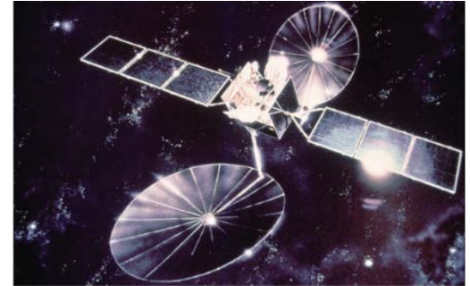
MSAT satellite used for cellular communications. Its satellite dishes allow cell signals to converge (focus) on the chosen coverage area. Credit: Communications Research Center Canada
